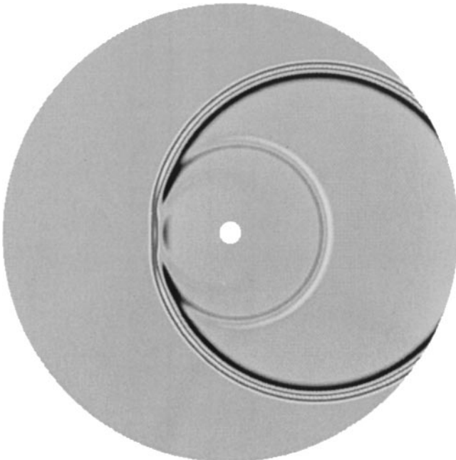
FIG. 10. Snapshot of pressure at time = 7.5 for 2-D linear wave.
